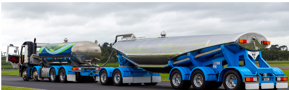
LONGVELD/ TRT 5-AXLE REAR STEER TRAILER BEING TESTED AT HAMPTON DOWNS BY FONTERRA
