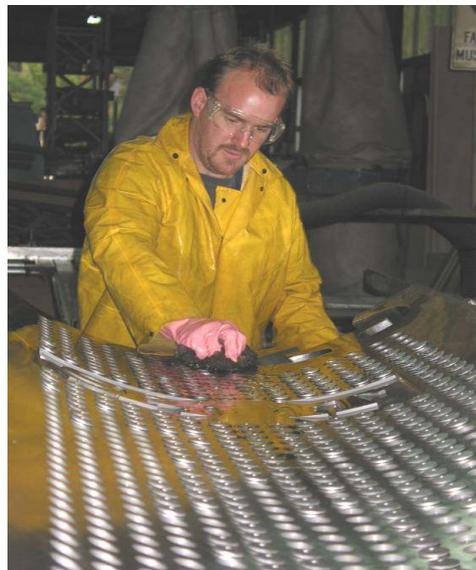
**Figure 2.** Left: *Type 316 stainless steel memorial. It has been finished with a vertical No.4 polish finish.*
